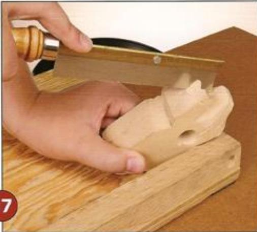
**Separate the Front Legs.** With the backsaw, cut between the front legs to separate them. Then, use the knife to shape them.
